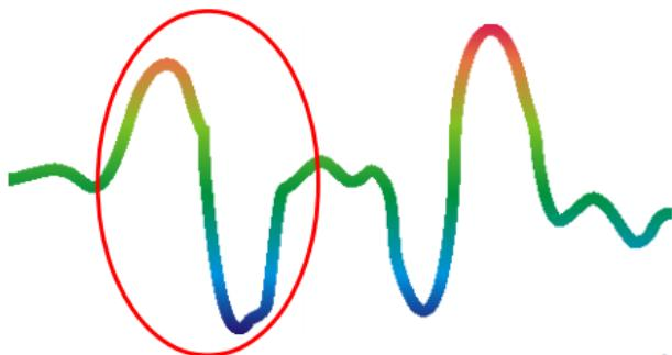
Figure 7.6: Signature of a ferromagnetic metal target
