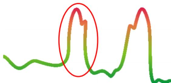
Figure 7.7: Signature of a non-ferromagnetic metal target
