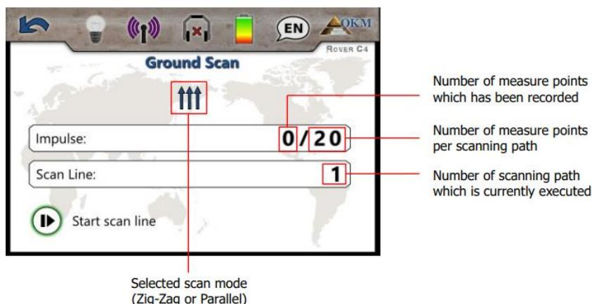
Figure 7.2: Display representation in operating mode "Ground Scan"
