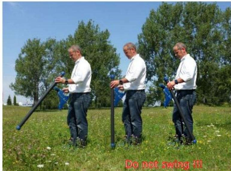
*Figure 7.5: Pinpointing with Super Sensor*
